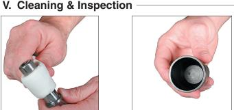
2. Inspect the Tube Assembly for any damage, especially around the mouth of the Tube Assembly. Lightly polish out any scratches at the mouth of the Tube Assembly to avoid damaging seals during the reassembly process. I damage to the Tube Assembly is severe it must be replaced. Wash, clean and dry the inside thoroughly.
