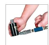
4. Slowly open the shut-off valve at the end of the charging hose and allow the gas spring to reach the desired charging pressure. You may also use the 90.310.044.
