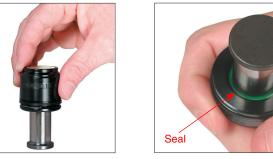
3. Be careful not to force the cartridge at an angle during assembly as the seal may get damaged. Once the Cartridge Assembly is installed, verify that the seal is properly aligned to the rod.
