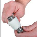
1. Lightly polish the rod surface with an emery cloth (600 grit). Inspect the finish of the rod for any scratches or gouges. If the rod is damaged it must be
