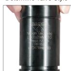
2. For the U Series proceed to Compact Valve Port, Step 3. For the L or LJ Series springs, examine the outside of the tube. An additional step in the tube indicates a Compact Valve port, proceed to Step 3.
