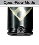
1. Check the port for deposits or burrs and clean thoroughly. Inspect the service fitting and replace if it shows signs of damage. Lubricate threads and seals on the fitting and thread the service fitting into the gas spring port.
