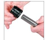
2. Once the cartridge and rod are removed from the Tube Assembly slide the cartridge off the rod and discard. Retain the rod for inspection and reuse.
