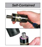
8. Install the new Dust Cover, (90.246.x.x). Tap with a soft mallet until the top of the Dust Cover rests flush with the top of the Tube Assembly. The rod wiper should be visible.
