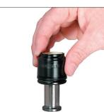
2. Position the new Cartridge Assembly over the rod, making sure that the wiper end marked "TOP" is facing up. While holding the cartridge vertically, slide the cartridge down the rod to the rod retainer
