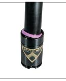
1. Stand the gas spring upright. Place a Removal Sleeve (90.340.x), longer than the stroke over the rod. Make sure to use the proper removal sleeve for the cylinder. Tap the sleeve until the Dust Cover, (90.246.x.x), is loosened. Remove the Dust Cover and discard.
