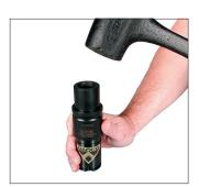
6. Insert the C-Style Retaining Ring in the retaining ring groove using a DADCO C-Ring Installation Tool, (90.351.x or 90.352). Be sure the C-Style Retaining Ring is fully seated in the retaining ring groove. For a detailed explanation of how to use the 90.352 C-Ring Installation Tool refer to bulletin #B01101E.
