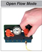
1. Exhaust nitrogen gas by opening the bleed valve on the control panel.
