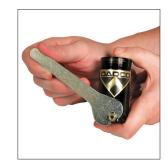
3. Unthread the service fitting and wipe with a clean cloth. Proceed to "II. Port Maintenance" Open Flow Mode, Step 1.
