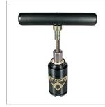
1. To remove the Rod and Cartridge Assembly thread a T-Handle, (90.320.M), into the rod end. Pull the entire assembly out of the tube. The spring body can be held in a vise (with soft jaws) while pulling out the assembly.
