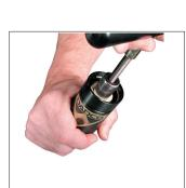
7. Thread the T-Handle, (90.320.M), into the end of the piston rod. Pull up on the T-Handle until the top of the cartridge is completely past the c-ring. The rod must seat the cartridge assembly fully before charging. The cartridge should be flush with the end of the cylinder. Make sure the rod is extended to its proper stroke length. (Depress the needle valve to facilitate full rod extension.)
