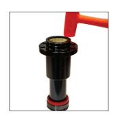
1. Install the Guide Rod into the Guide Retainer using a soft rubber mallet.
