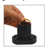
2. Remove the bottom bushing from the Guide Retainer using a small screwdriver and discard.
