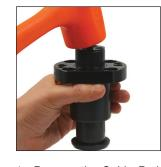
Remove the Guide Rod from the Guide Retainer using a soft rubber mallet. A vise, with soft jaws, may be used to secure the Guide Retainer if needed.
