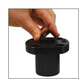
6. Install the new wiper into the top of the Guide Retainer. Check to see it is well seated.
