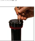
12. Install the safety wire ring onto the Rod Retainer by hand using a small screw driver to make sure it properly seats into the groove.
