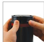
3. Remove the two halves of the rod retainer from the Guide Rod and retain for reassembly.
