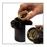
7. Install the top bushing (yellow) by overlapping the gap portion and placing it below the wiper into the Guide Retainer. The bushings may not seat properly if the wiper is not seated properly.
