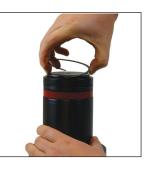
5. Install the rod retainer ring
