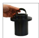
3. Remove the two middle bushings from the guide retainer. Discard used bushings. Inspect the Guide Retainer for any damage. Wash and dry the inside thoroughly.
