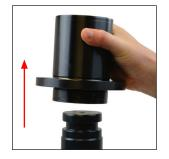
5. Pull the Guide Retainer off the Guide Rod. You may need to use a soft rubber mallet. A vise, with soft jaws, may be used to secure the Guide Rod
