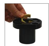
4. Remove the top bushing from he Guide Retainer using a small screwdriver and discard.
