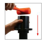
1. Using a soft rubber mallet install the Guide Retainer onto the Guide Rod.
