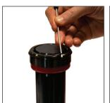
Rod Retainer using a small retain for reassembly. screwdriver. Retain the ring for reassembly.
