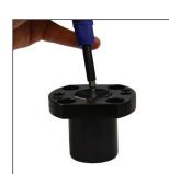
5. Remove the rod wiper using a small screwdriver and discard. Then remove the middle bushing. Inspect the Guide Retainer for any damage. Wash and dry the inside thoroughly.
