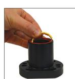
9. Install the third new bushing into the bottom of Guide Retainer. To insert, overlap the gap portion and push the bushing into place past the excluder/dampener. Once all the bushings are installed, use all the grease supplied in the kit to grease the bushings.
