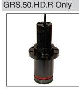
1. Remove the guide rod adapter cap located at the top of the GRS.50.HD.R Guide Rod, using a 5 mm allen wrench to unthread the cap screw.
