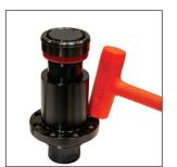
1. Remove the Guide Rod from the Guide Retainer using a soft rubber mallet. A vise, with soft jaws, may be used to secure the Guide Retainer if needed.
