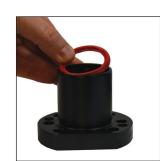
8. Install the new excluder/ dampener into the bottom of Guide Retainer. Check to see it is well seated.
