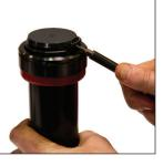
on the Guide Rod using a soft ring using a small screwdriver dampener to remove it from the from the Guide Rod. If needed, or external snap ring spreaders. Guide Rod, and discard. If needed, a vise, with soft jaws, may be used to secure the Guide Rod. Retain the ring for reassembly.
