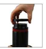
2. Remove the guide rod retaining key by sliding it off the Guide Rod. Retain the key for reassembly
