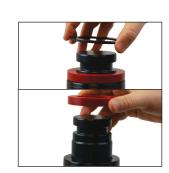
4. Remove the dampener backing ring and then the dampener from the Guide Rod. Retain the ring for reassembly and dispose of the dampener.
