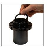
6. Install a new wiper into the top of Guide Retainer. Check to see it is well seated.
