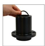
5. Install the bottom wiper (if it was present in step 1), then install the bottom bushing (black) by overlapping the gap portion and placing it into the Guide Retainer.
