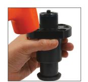
10. Install the Guide Rod into the Guide Retainer using a soft rubber mallet.
