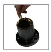
1. Remove the bottom bushing from the guide retainer using a small screwdriver. Then remove the bottom wiper (if present). Discard used bushing.
