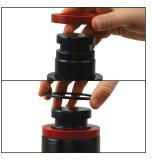
2. Install the dampener and then the dampener backing ring on to the Guide Rod.
