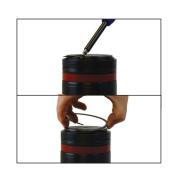
1. Remove the rod retainer ring located at the bottom of the guide rod using a screwdriver. Retain ring for reassembly
