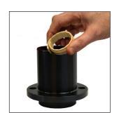
4. Install the two new middle (yellow) bushings one at a time by overlapping the gap portion and placing them into the Guide
