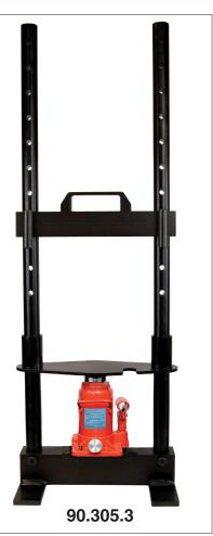
Note: 90.305.3 dimensions are *H* = 991 *mm*, *W* = 305 *mm*, *D* = 229 *mm* Not designed for use as an arbor press.
