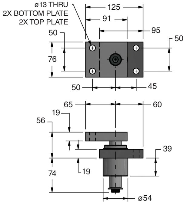
**Note:** Guide Rod Assembly for use with the Single Post Direct Lift only.
