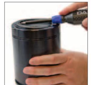
2. Using the Port Servicing Tool, (90.320.8), pry the Wiper Retainer from the top of the gas spring and retain for reassembly.
