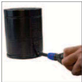
2S. Remove the Compact Valve, (90.260), by unscrewing it with the Port Servicing Tool, (90.320.8). Thread a new Compact Valve, (90.260), into the port until it fits snugly on the seat. Avoid over torquing the valve.
