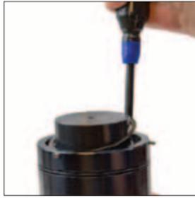
10. Insert the Spirolox Retaining Ring in the retaining ring groove using the Port Servicing Tool, (90.320.8). Be sure the Spirolox Retaining Ring is fully seated in the groove.
