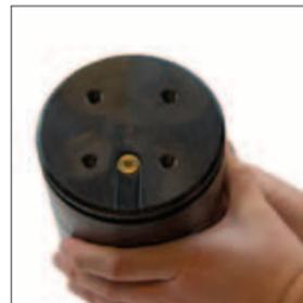
1. Visually inspect the rupture disk located at the bottom of the gas spring for damage. If damaged, remove with the Port Servicing Tool, (90.320.8), and replace with a new rupture disk (RD-400G).
