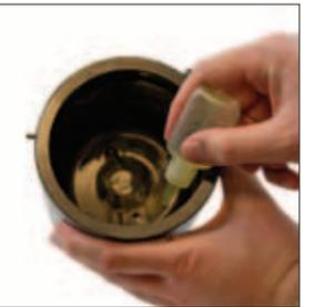
6. Lubricate the inside wall of the Tube Assembly with all remaining DADCO Assembly Oil.
