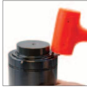
11. Install the Wiper Retainer. Tap with a soft mallet until the top of the Wiper Retainer rests flush with the top of the can. The rod wiper should be visible.
