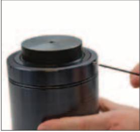
11. Using a 2 mm allen wrench, tighten the three set screws at the top of the gas spring.
