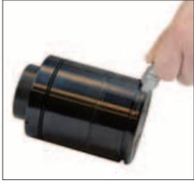
1S. Thread the Quick Disconnect Charging Nipple, (90.310.111), into the port of the gas spring. Connect the female end of the charging assembly to the charging nipple and pressurize the gas spring. Do not exceed the maximum charging pressure of 150 bar (2175 psi). The DADCO Pressure Analyzer, (90.315.5), can also be used for charging, discharging and gauging pressure in self-contained gas springs.
