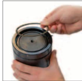
2. Continue moving around the Spirolox Retainer Ring until removed. Keep the ring for reassembly.
