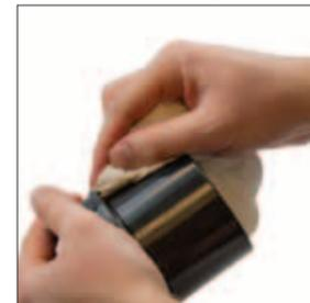
1. Lightly polish the rod surface with an emery cloth (600 grit). Inspect the seal groove for any scratches or gouges. If the groove is damaged then the rod must be replaced.
