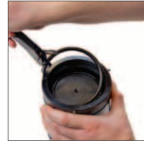
5. Once the hooked end of the tool is firmly seated below the c-ring, begin pushing it toward the outside of the gas spring can. The handles will close naturally, and the c-ring will be extracted as you complete this motion. For a detailed explanation of c-ring removal see bulletin B15127A.
