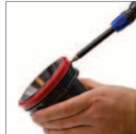
4. Remove the Seal from the Rod Retainer using the Port Servicing Tool, (90.20.8), and discard. Be careful not to scratch the rod.
