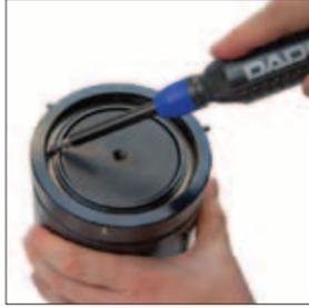
1. Using the Port Servicing Tool, (90.320.8), start at the tab and begin to pry up the Spirolox Retainer Ring.
