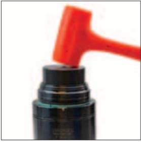
7. Place the rod and cartridge into the Tube Assembly. Use the Valve Bleed Tool, (90.360.4), or Port Servicing Tool, (90.320.8), to depress the valve to release any back pressure. Position the top of the cartridge just below the retaining ring groove.
