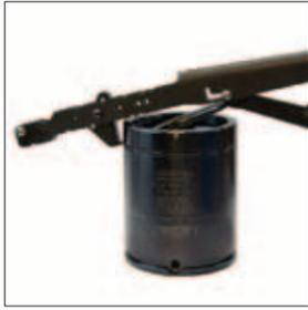
8. Insert the C-Style Retaining Ring in the retaining ring groove using a DADCO C-Ring Installation Tool, (90.352). Be sure the C-Style Retaining Ring is fully seated in the retaining ring groove. For a detailed explanation of c-ring installation, see bulletin B01101D.
