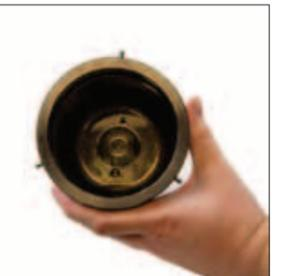
2. Inspect the Tube Assembly for any damage, especially around the mouth of the Tube Assembly. Lightly polish out any scratches at the mouth of the Tube Assembly to avoid damaging seals during the reassembly process. If damage to the Tube Assembly is severe it must be replaced. Wash, clean and dry the inside thoroughly.
