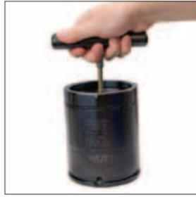
9. Thread the T-Handle, (90.320.1 or 90.320.2), into the end of the piston rod. Pull up on the T-Handle until the top of the cartridge is completely past the c-ring.
