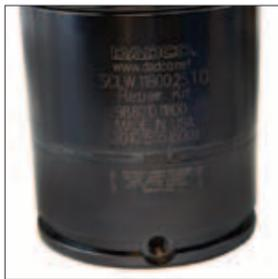
1S. Generally the valve does not need replacing. Only if the valve appears damaged, is leaking pressure or sticking proceed to step 2S, otherwise leave the valve undisturbed and proceed to "III. Rupture Disk."
