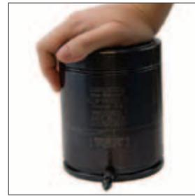
4. After all the gas pressure is exhausted, be sure that the piston rod will freely retract into the tube manually. If not, try depressing the valve again. If still unsuccessful **STOP** and contact DADCO.
