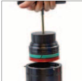
1. To remove the Rod and Cartridge Assembly thread a T-Handle, (90.320.1 or 90.320.2), into the rod end. Pull the entire assembly out of the Tube Assembly. The spring body can be held in a vise (with soft jaws) while pulling out the assembly.
