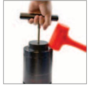
12. Thread the T-Handle, (90.320.1 or 90.320.2), into the end of the piston rod. Pull up on the T-Handle to verify the cartridge is completely past the c-ring. The rod must seat the cartridge assembly fully before continuing. Make sure the rod is extended to its proper stroke length. (If needed, depress the valve to facilitate full rod extension.)
