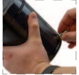
1L. Install the fitting into the port and pipe all gas springs back to the control panel, making sure that all connections are tight and that gas spring rods are extended.
