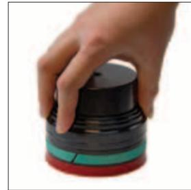
4. Slide the Cartridge Assembly onto the rod, making sure that the wiper end marked "TOP" is facing up.
