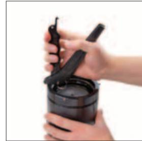
4. Remove the C-Style Retaining Ring, (90.285.80.x.), using the C-Ring Removal Tool, (90.356). Position the hooked end of the tool below the c-ring. For best results locate the tool near either end of the c-ring.
