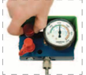
2L. Attach Charging Assembly (90.310.040) to the quick disconnect filler valve on the control panel and pressurize the system. Do not exceed the maximum charging pressure of 150 bar (2175 psi).
