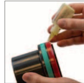
5. Lubricate the seal with a few drops of the DADCO Assembly Oil, included in the seal kit.
