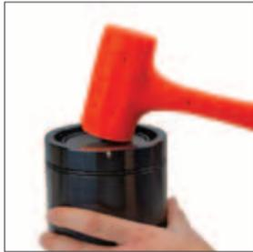
3. Tap the top of the rod until the rod and housing are below the retaining ring groove.
