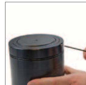
1. Using a 2 mm allen wrench, unthread the three set screws at the top of the gas spring, but keep them installed. The set screws are easily lost if removed completely.
