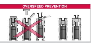
Jammed parts are very dangerous. If parts are jamming, determine the root cause and repair it before production continues. Slight pre-load of gas spring prevents damage from sudden release. Sudden release may damage and / or vent cylinders.
