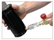
2. Charge the gas spring with nitrogen gas to the preset value plus at least 20 bar/2 MPa, refer to Page 1 for more information.
