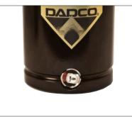
When the nitrogen pressure in the gas spring is below the preset value the Compact Pressure Indicator displays red. The indicator cannot be reset until the gas spring is charged.
