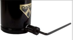
2. Place the removal tool over the Compact Pressure Indicator and align the teeth of the removal tool with the grooves of the indicator. Use the allen wrench to turn the removal tool, loosening the indicator from the gas spring.
