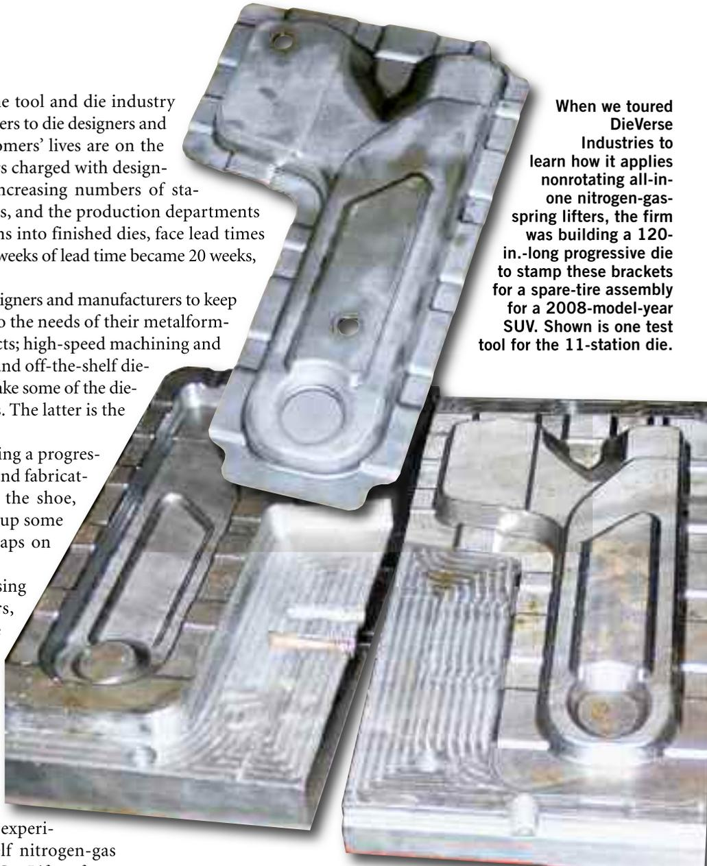
When we toured DieVerse Industries to learn how it applies nonrotating all-in-one nitrogen-gas-spring lifters, the firm was building a 120-in.-long progressive die to stamp these brackets for a spare-tire assembly for a 2008-model-year SUV. Shown is one test tool for the 11-station die.
