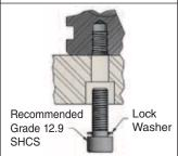
Use a serviceable thread locking compound and lock washers when installing socket head cap screws.
