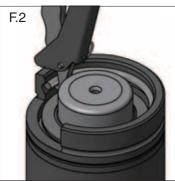
2. HOOKING: Position the claw end of the C-Ring Removal Pliers below the C-Ring. For best results hook the C-Ring about 6 mm or .25" from either end of the C-Ring (F.2). Be careful not to damage the gas spring rod. Ring may be removed in horizontal or verticle position.
