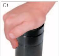
1. Follow the maintenance instructions to discharge the gas spring pressure. Verify that the gas pressure has been exhausted by pushing the piston rod down manually. The rod will freely retract into the tube (F.1). If unsuccessful pushing down the rod completely then **STOP** and contact DADCO. To Access the C-Ring, remove the dust cover and push the rod cartridge below the C-style Retaining Ring groove.
