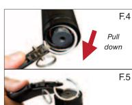
4. PRYING: To pry the C-Ring out, use the notched end of the pliers as a lever against the top edge of the can (F.4). For larger models the tool may need to be reset to reposition the notched end of the tool.
