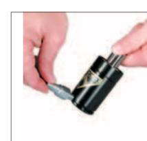
1. To increase the spring pressure, thread the Quick Disconnect Filler Valve, (90.310.143), into the port, set the regulator to the desired pressure and fill. The 90.315.5 may also be used to adjust pressure.
