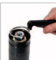
3. Remove the C-style Retaining Ring, (90.285.x.x), using a C-Ring Removal Tool, (90.355). Position the hooked end of the tool below the c-ring. For best results locate the tool near either end of the c-ring. (Use the Port Servicing Tool to pry out C-style Retaining Rings found in 13 mm stroke or shorter models.)
