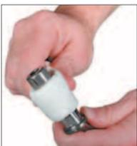
1. Lightly polish the rod surface with an emery cloth (600 grit). Inspect the finish of the rod for any scratches or gouges. If the rod is damaged it must be replaced.
