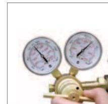
3. Set the desired charging pressure on the regulator. DADCO recommends charging the spring to the maximum charging pressure of 150 bar (2175 psi).
