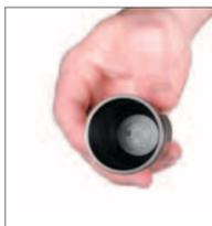
2. Inspect the Tube Assembly for any damage, especially around the mouth of the Tube Assembly. Lightly polish out any scratches at the mouth of the Tube Assembly to avoid damaging seals during the reassembly process. If damage to the Tube Assembly is severe it must be replaced. Wash, clean and dry the inside thoroughly.
