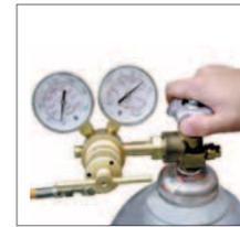
2. Open the main valve on the nitrogen tank.
