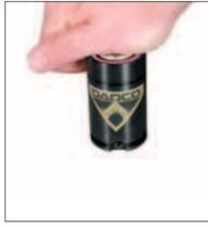
4. After all of the gas pressure is exhausted, be sure that the piston rod will freely retract into the tube manually. If not, try depressing the valve again. If still unsuccessful **stop** and contact DADCO.
