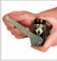
3. Unthread the service fitting and wipe with a clean cloth. Proceed to "II. Port Maintenance" *Open Flow Mode*, Step 1.
