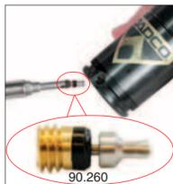
4A. Thread a new Compact Valve, (90.260), into the port until it fits snugly on the seat. Avoid over torquing the valve.
