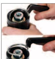
4. Once the hooked end of the tool is firmly seated below the c-ring, begin pushing it toward the outside of the gas spring tube. The handles will close naturally, and the c-ring will be extracted as you complete this motion. For a detailed explanation of c-ring removal see bulletin #B13113A.
