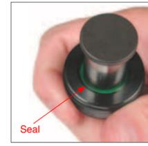
3. Be careful not to force the cartridge at an angle during assembly as the seal may get damaged. Once the Cartridge Assembly is installed, verify that the seal is properly aligned to the rod.
