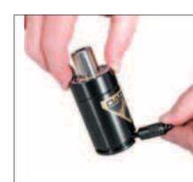
2. To decrease the gas spring pressure, depress the valve stem using a DADCO Valve Bleed Tool, (90.360.4).
