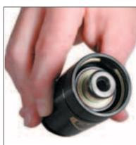
2. Reposition the DADCO Removal Sleeve and only continue tapping until the rod, cartridge assembly is slightly below the retaining ring groove. The bore of the Tube Assembly is designed to stop the cartridge in this position. **DO NOT force the cartridge down further into the Tube Assembly.**
