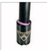
1. Stand the gas spring upright. Place a Removal Sleeve (90.340.x), longer than the stroke over the rod. Make sure to use the proper removal sleeve for the cylinder. Tap the sleeve until the Dust Cover, (90.246.x.x), is loosened. Remove the Dust Cover and discard.
