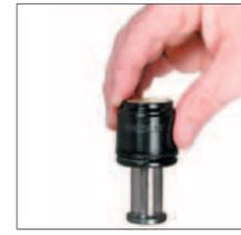
2. Position the new Cartridge Assembly over the rod, making sure that the wiper end marked "TOP" is facing up. While holding the cartridge vertically, slide the cartridge down the rod to the rod retainer.
