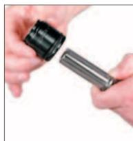
2. Once the cartridge and rod are removed from the Tube Assembly slide the cartridge off the rod and discard. Retain the rod for inspection and reuse.
