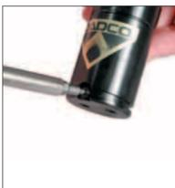
5B. Retrieve and replace the Valve Retaining Screw, (90.251). Proceed to step "III. C-Ring Removal."
