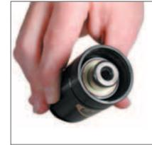
5. Place the rod and cartridge into the Tube Assembly. Depress the needle valve to release any back pressure. Position the top of the cartridge just below the retaining ring groove. The bore of the cartridge assembly is designed to stop the cartridge in this position. **DO NOT force the cartridge down further into the tube.**
