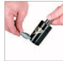
1. Thread the M6 end of the Quick Disconnect Filler Valve, (90.310.143), into the port of the gas spring. Connect the female end of the charging assembly to the charging nipple. The DADCO Pressure Analyzer, (90.315.5), can also be used for charging, discharging and gauging pressure.
