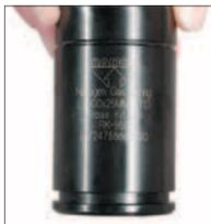
2. For the U Series proceed to *Compact Valve Port*, Step 3A. For the L or LJ Series springs, examine the outside of the tube. An additional step in the tube indicates a Compact Valve port, proceed to *Compact Valve Port*, Step 3A. If there is no additional step in the tube then proceed to *Tire Valve Port*, Step 3B.
