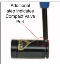
3A. Remove the Compact Valve, (90.260), by unthreading it with the Port Servicing Tool, (90.320.8).
