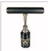
1. To remove the Rod and Cartridge Assembly thread a T-Handle, (90.320.7 or 90.320.2), into the rod end. Pull the entire assembly out of the tube. The spring body can be held in a vise (with soft jaws) while pulling out the assembly.
