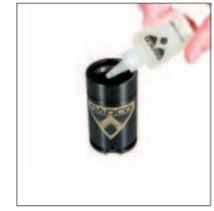
4. Lubricate the inside wall of the tube with the DADCO Assembly Oil.
