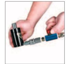
4. Slowly open the shut-off valve at the end of the charging hose and allow the gas spring to reach the desired charging pressure. You may also use the 90.310.044.
