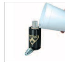
7. Check for leaks at the top of the tube around the rod and at the base around the valve compartment using mineral oil or water. Verify the pressure with a DADCO Load Cell using a DADCO Portable Test Stand, (90.305.3). **NOTE: If spring is open-flow, the filler valve (90.310.143) must remain in place during testing.**
