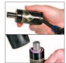
8. Install the new Dust Cover, (90.246.x.x). Tap with a soft mallet until the top of the Dust Cover rests flush with the top of the Tube Assembly. The rod wiper should be visible.
