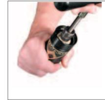
7. Thread the T-Handle, (90.320.7) or (90.320.2), into the end of the piston rod. Pull up on the T-Handle until the top of the cartridge is completely past the c-ring. The rod must seat the cartridge assembly fully before charging. The cartridge should be flush with the end of the cylinder. Make sure the rod is extended to its proper stroke length. (Depress the needle valve to facilitate full rod extension.)
