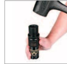
6. Insert the C-Style Retaining Ring in the retaining ring groove using a DADCO C-Ring Installation Tool, (90.351.x or 90.352). Be sure the C-Style Retaining Ring is fully seated in the retaining ring groove. For a detailed explanation of how to use the 90.352 C-Ring Installation Tool refer to bulletin #B01101D.
