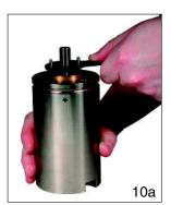
(9) Grease the piston rod with a small amount of hydraulic fluid. Twist the new cartridge while sliding it onto the rod.(10a) Using a spanner wrench, turn the front cartridge until it rests flush with the top of the cylinder.
