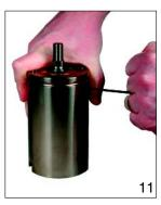
(10b) For the double rod end model, completely reinstall the front cartridge then repeat steps 9 and 10a for the rear head.
