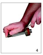
(3) Pull the entire rod assembly out of the cylinder. Once the assembly is removed, slide the rod cartridge off the rod and discard. (4) Remove the old piston seal. Take care not to scratch the finish on the piston rod.
