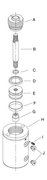
\* Must also specify stroke length when ordering these parts. Repair Kits DK40-RK and DK55-RK include items A & D Repair Kits DKD40-RK and DKD55-RK include items A, D & K
