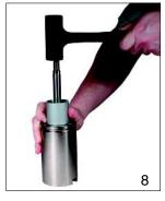
(6) Insert the starter tube into the cylinder.(7) Slide the piston rod assembly into the cylinder.(8) Using a soft mallet, tap the piston rod assembly until the piston reaches the bottom of the cylinder.Remove the starter tube.
