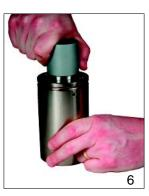
(5) Install the new piston seal. The soft o-ring seal should be installed first. The outer seal should then be installed with a small, flat blade screwdriver. Take care not to damage the seal. The outer seal may be made more pliable by heating in warm oil.
