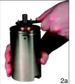
(1) Loosen the set screw(s) by turning counterclockwise 1-2 turns. (2a) Using a spanner wrench, unscrew the front head rod cartridge. (2b) For the double rod end model, unscrew and remove the rear head cartridge.
