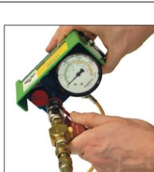
2L. Attach Charging Assembly (90.310.040 or 90.310.045) to quick disconnect filler valve on the control panel.
