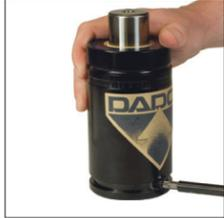
3. Replace damaged Cartridge Valve. Use Port Servicing Tool (90.320.8) to thread new Cartridge Valve into the port until it fits snugly on the seat. Avoid over torquing the valve.
