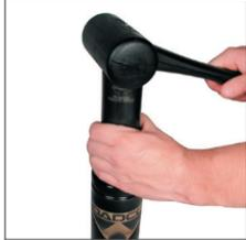
1. Stand gas spring upright. Make sure rod is retracted in tube. Place Removal Sleeve (90.340.x) over rod. Tap sleeve until Dust Cover (90.246.x) is loosened. Remove dust cover and discard.
