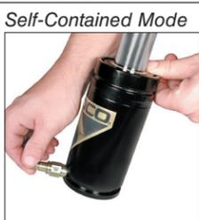
1S. Thread the Quick Disconnect Charging Nipple (90.310.111) into the port. Connect the female end of the Charging Assembly (90.310.040 or 90.310.045) to the charging nipple. The DADCO Pressure Analyzer (90.315.5) may also be used.
