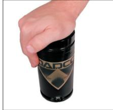
4. After all gas pressure is exhausted, be sure piston rod will freely extend and retract into tube manually. If not, try depressing valve again. If still unsuccessful, **STOP** and contact DADCO.
