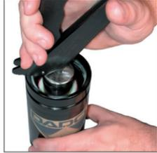
3. Remove C-style Retaining Ring (90.285.x) using C-Ring Removal Tool (90.356). Position correct hooked end of C-Ring Removal Tool below c-ring. For best results locate tool near either end of c-ring.
