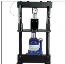
8. Verify pressure with a DADCO Load Cell using a DADCO Portable Test Stand (90.305.3) or an arbor press.
