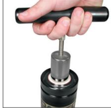
7. Thread T-Handle (90.320.2) into end of piston rod. Pull up on t-handle until top of cartridge is past c-ring. The rod must seat cartridge assembly fully (with the housing flush with end of cylinder). Make sure rod is extended to its proper stroke length. (Depress cartridge valve to facilitate full rod extension.)
