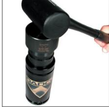
4. Thread assembly cap onto rod. Place rod and cartridge assembly into spring. To release any back pressure, depress cartridge valve. Position top of cartridge just below retaining ring groove. Tap assembly cap to drive rod and cartridge assembly into tube assembly.
