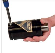
2. Remove Port Plug (90.505.110) located at the base of the spring. Retain parts for use during reassembly.
