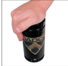
2. Verify all pressure is relieved by manually retracting piston rod into tube. If rod will not fully retract, release remaining pressure. If still unsuccessful, **STOP** and contact DADCO.
