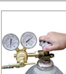
3. Open main valve on nitrogen tank.
