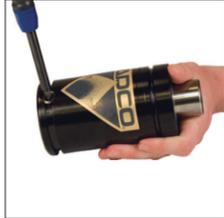
3. Keeping face and hands clear of port, use Valve Bleed Tool (90.360.4) or Port Servicing Tool (90.320.8) to depress Cartridge Valve (90.265). Cover port with a cloth to absorb discharge.
