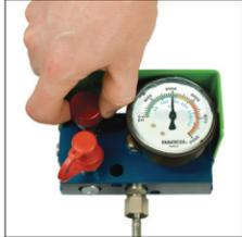
1. Exhaust nitrogen gas by opening bleed valve on the control panel.
