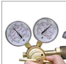
1S. To increase spring pressure, thread the Quick Disconnect Charging Nipple (90.310.111) into the port, set the regulator to the desired pressure and fill. DADCO's Pressure Analyzer (90.315.5) may also be used to adjust pressure.
