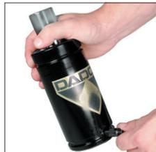
2S. To decrease gas spring pressure, depress valve stem using a DADCO Valve Bleed Tool (90.360.4).
