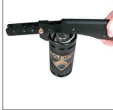
6. Insert C-Style Retaining Ring (90.285.x) into retaining ring groove using C-Ring Installation Tool (90.350.00750 or 90.352) or standard bench tools. Be sure C-Style Retaining Ring is fully seated in retaining ring groove.
