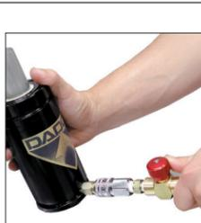
6. Disconnect charging assembly from control panel. The small amount of nitrogen trapped between the shut-off valve and filler valve will bleed off as you disconnect fitting.
