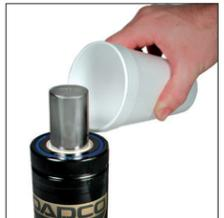
7. Check for leaks at top of tube around rod and at base around valve compartment using vegetable oil.
