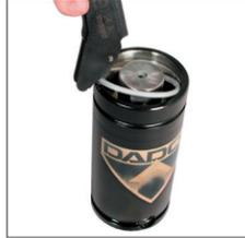
4. Once hooked end of tool is firmly seated below c-ring, begin pushing it toward outside of gas spring can. The handles will close naturally and c-ring will be extracted as you complete this motion.
