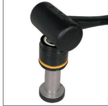
2. Position cartridge assembly over the rod, making sure wiper end marked "TOP" is facing up. While holding cartridge vertically, slide it down the rod to the rod retainer. Be careful not to force cartridge at an angle as seal could become damaged.
