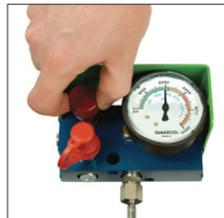
1L. To increase system pressure, set regulator on nitrogen tank to desired level and fill system through control panel. To release pressure, open drain valve on control panel.
