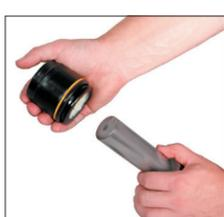
3. Once cartridge and rod are removed from tube assembly, slide cartridge off of rod and discard. Retain rod for inspection and possible reuse.
