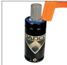
10. Install new Dust Cover (90.246.5B.x). Tap with a soft mallet until top of Dust Cover rests flush with top of can.
