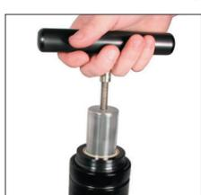
1. To remove cartridge assembly, thread a T-Handle (90.320.2) into the rod end.
