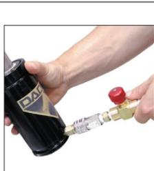
5. Slowly open shut-off valve and allow gas spring to reach desired charging pressure. After charging, CLOSE HOSE SHUT-OFF VALVE AND TANK SHUT-OFF VALVE.
