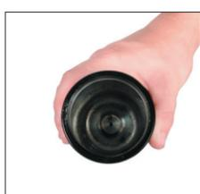
2. Inspect tube assembly for damage, especially around opening. Polish scratches at mouth of tube assembly to avoid damaging seals during reassembly. If damage to tube assembly is severe, it must be replaced.
