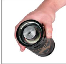
2. Reposition removal sleeve and continue tapping until rod cartridge assembly is slightly below retaining ring groove. DO NOT force the cartridge down further into the Tube Assembly.
