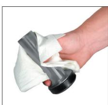
1. Lightly polish rod surface with emery cloth (600 grit). Inspect finish of rod for scratches or gouges. If rod is damaged, it must be replaced. If present, rod safety ring should remain in place.
