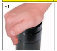
1. Follow the maintenance instructions to discharge the gas spring pressure. Verify that the gas pressure has been exhausted by pushing the piston rod down manually. The rod will freely retact into the tube (F.1). If unsuccessful pushing down the rod completely then **STOP** and contact DADCO. To Access the C-Ring, remove the dust cover and push the rod cartridge below the C-style Retaining Ring groove.\*
