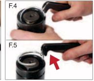
4. PRYING: To pry the C-Ring out, use the end of the pliers as a lever against the top edge of the can (F.4). The tool may need to be rocked back and forth several times to pry out the C-ring.
