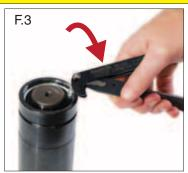
3. LIFTING: Once the hooked end of the tool is firmly seated below the C-Ring, begin pushing the pliers down to lift the C-Ring from the groove. The handles will close naturally as you complete this motion (F.3).
