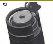
2. HOOKING: Position the claw end of the C-Ring Removal Pliers below the C-Ring. For best results hook the C-Ring about 6 mm or .25" from either end of the C-Ring (F.2). Be careful not to damage the gas spring rod. Models 400 through 750 have limited room between the tube and rod; be careful when capturing the C-Ring. The tool may need to be slid through the gap in the C-Ring and slid sideways underneath the C-Ring to position correctly.
