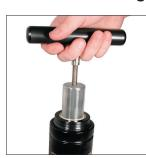
1. To remove the Cartridge Assembly, thread a T-Handle (90.320.M) into the rod end.
