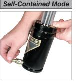
1S. Thread the Quick Disconnect Charging Nipple (90.310.111) into the port of the gas spring. Connect the female end of the Charging Assembly (90.310.040 or 90.310.045) to the charging nipple. The DADCO Pressure Analyzer (90.315.5) can also be used for charging, discharging and gauging the pressure.
