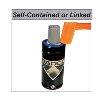
10. Install the new Dust Cover (90.246.x). Tap with a soft mallet until the top of the Dust Cover rests flush with the top of the can. The rod wiper should be visible.
