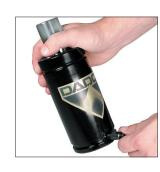
2S. To decrease gas spring pressure, depress the valve stem using a Valve Bleed Tool (90.360.4).
