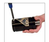
2. Remove the Port Plug (90.505.110) located at the base of the spring. Retain parts for use during reassembly.
