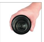
2. Inspect the Tube Assembly for any damage, especially around the mouth of the Tube Assembly. Polish out any scratches at the mouth of the tube assembly to avoid damaging seals during the reassembly process. If damage to the Tube Assembly is severe
