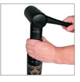
1. Stand the gas spring upright Make sure the rod is retracted in the tube. Place a Removal Sleeve (90.340.x) over the rod. Tap the sleeve until the Dust Cover (90.246.x) is loosened. Remove the Dust Cover and discard.
