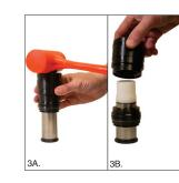
3A. While holding the cartridge, vertically tap the Assembly Cap to drive the cartridge down the rod. Be careful not to force the cartridge at an angle as the seal could become damaged.
