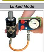
1L. Pipe all gas springs back to the control panel, making sure that all connections are tight and that gas spring rods are extended.
