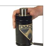
3. Replace the damaged valve. Use the Port Servicing Tool (90.320.8) to thread the new valve into the port until it fits snugly on the seat. Avoid over torquing the valve.
