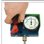
1. Exhaust nitrogen gas by opening the bleed valve on the control panel.
