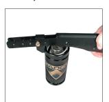
7. Insert the C-Style Retaining Ring (90.285.x) in the retaining ring groove using a DADCO C-Ring Installation Tool (90.350.x, 90.351.x or 90.352) or standard bench tools. Be sure C-Style Retaining Ring is fully seated in retaining ring groove.
