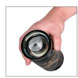
2. Reposition the Removal Sleeve and continue tapping until the rod cartridge assembly is slightly below the Retaining Ring groove. DO NOT force the cartridge down further into the Tube Assembly.
