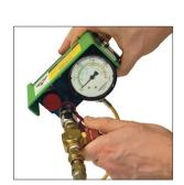
2L. Attach Charging Assembly (90.310.040 or 90.310.045) to the quick disconnect filler valve on the control panel.
