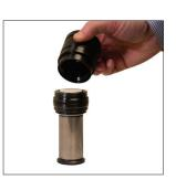
2. Thread Assembly Cone (90.331.x) from Cartridge Starter Kit (90.335.x) onto rod. Slide Cartridge Assembly over the Assembly Cone, making sure that the wiper end marked "TOP" is facing up. Place Cartridge Assembly Cap (90.330.x) from Cartridge Starter Kit (90.335.x) on top of Cartridge Assembly.
