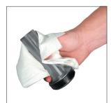
1. Lightly polish the rod surface with an emery cloth (600 grit). Inspect the finish of the rod for any scratches or gouges. If the rod is damaged it must be replaced. If present, the Rod Safety Ring should remain in place.
