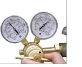
1S. To increase spring pressure, thread the Quick Disconnect Charging Nipple (90.310.111) into the port, set the regulator to the desired pressure and fill. DADCO's Pressure Analyzer (90.315.5) may also be used to adjust pressure.
