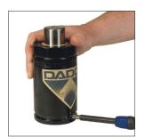
2. Remove valve using the Port Servicing Tool (90.320.8). Compact Valve (90.260) requires a T20 drive or bit, Cartridge Valve (90.265) requires a T40 drive or bit.
