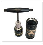
2. Pull the entire assembly out of the tube. Depress the cartridge valve to relieve any back pressure.
