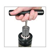
8. Thread T-Handle (90.320.M) into the end of the piston rod. Pull up on T-Handle until the top of the cartridge is past the c-ring. The rod must seat cartridge assembly fully (with the housing flush with end of cylinder). Make sure rod is extended to its proper stroke length. (Depress cartridge valve to facilitate full rod extension.)
