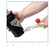
5. Slowly open the shut-off valve and allow gas spring to reach the desired charging pressure. After the gas spring has been charged to the desired pressure, CLOSE THE HOSE SHUT-OFF VALVE AND THE TANK SHUT-OFF VALVE.
