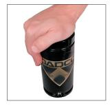
2. Verify that all pressure is relieved by manually retracting the piston rod into the tube. If the rod will not fully retract release the remaining pressure. If still unsuccessful, STOP and contact DADCO.
