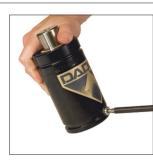
9S. Make sure the valve is in place and thread Port Plug (90.505.110) securely over top.
