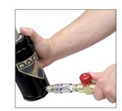
6. Disconnect the charging assembly from the charging nipple. The small amount of nitrogen trapped between the shut-off valve and filler valve will bleed off as you disconnect the fitting.
