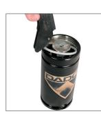
4. Once the hooked end of the tool is firmly seated below the c-ring, begin pushing it toward the outside of the gas spring can. The handles will close naturally, and the c-ring will be extracted as you complete this motion.
