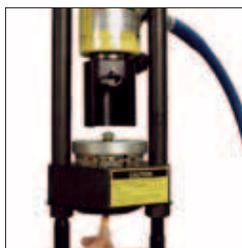
4. Position the hose and adapter into the crimp die from below.
