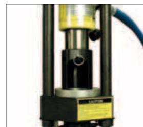
6. Actuate until the die ring contacts the base plate. **CAUTION: Keep hands clear of Karrykrimp machine during operation.**
