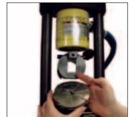
2. Place the crimp die into the base cavity. Note: The crimp dies are color-coded by size for easier identification.
