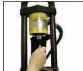
1. Remove the pin from the pusher in the Karrykrimp Machine and move the pusher back.
