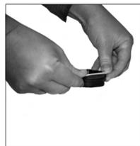
4. Place the rear head so the mounting holes are facing down. Install the O-Ring Backup, (98.249.80.x), and then the O-Ring, (98.245.80.x). The o-ring will be seated above the o-ring backup in the same groove. Verify that the o-ring backup and the o-ring do not twist when installing.
