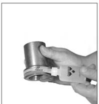
3. Once the new seal is pressed down evenly and positioned properly around the rod then snap the new piston rider around the rod. Lubricate the seal using the DADCO Assembly Oil and reinstall the rod assembly.
