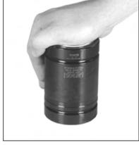
4. After all the gas pressure is exhausted remove the gas spring from the vise, be sure that the piston rod will freely retract into the tube manually. If not, try depressing the valve again. If still unsuccessful **STOP** and contact DADCO.
