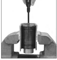
3. Keeping face and hands clear of the port, use the Valve Bleed Tool, (90.360.4), or the Port Servicing Tool, (90.320.8), to depress the Compact Valve (90.260). Cover the port with a cloth to absorb discharge.
