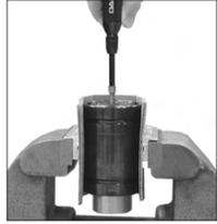
2. Remove the port plug, and sealing washer, (90.505.110), located on the bottom of the spring with the Port Servicing Tool, (90.320.8). Retain parts for use during reassembly.
