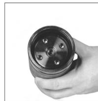
5. Reinstall the rear head into the tube. If necessary, depress the valve to release any back pressure.
