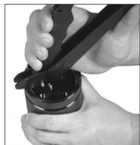
2. Remove the C-Style Retaining Ring, (98.285.80.x), using the C-Ring Removal Tool, (90.355 or 90.356). Position the hooked end of the C-Ring Removal Tool below the c-ring. For best results locate the tool near either end of the c-ring.
