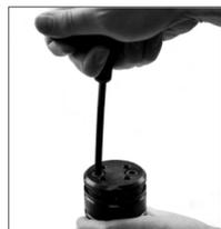
1. Remove the cap screws with washers from the bottom of the subplate and keep for reassembly.
