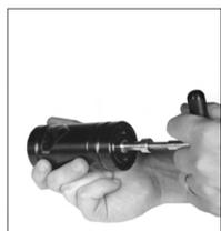
7. Thread DADCO's Rear Head Tool (90.320.1 or 98.328) into the port and pull out to seat the rear head against the c-ring.
