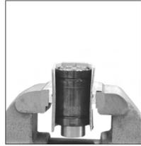
1. When exhausting pressure, position the gas spring upside down in a vise so that the cylinder is secured. Be sure to wrap the spring in cardboard to protect it from the vise.
