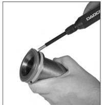
2. Remove the seal and piston rider. Pry the seal off the rod using the Port Servicing Tool, (90.320.8), be careful not to scratch the inside of the groove. Discard the seal and piston rider.
