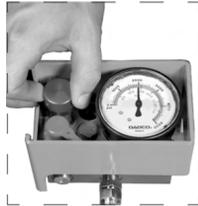
1. Exhaust nitrogen gas by opening the bleed valve on the control panel.
