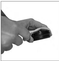
3. Using a small screwdriver, remove the O-Ring Backup, (98.249.80.x), and the O-Ring, (98.245.80.x), from the rear head, be careful not to scratch the inside of the groove. Discard both o-rings.
