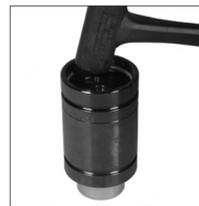
1. Hold the discharged gas spring upside down. Using a rubber mallet gently tap the rear head down into the tube. It may be necessary to depress the valve stem again to release any back pressure.
