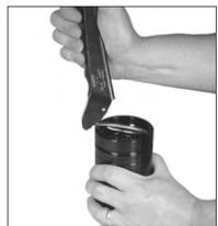
3. Once the hooked end of the tool is firmly seated below the c-ring, begin pushing it toward the outside of the gas spring can. The handles will close naturally, and the c-ring will be extracted as you complete this motion. Request the C-Ring Removal Tool Bulletin for more information.
