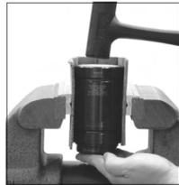
1. Wrap the cylinder in cardboard and place in a vise. With a soft rubber mallet, tap the rod down through the tube. This will push the rear head out at the same time. **Note:** You will need to guide the parts as they are pushed out. To avoid damaging the piston rod or bore do not let them drop onto a hard surface.
