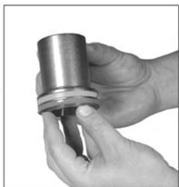
2B. Press the new seal down evenly until it is positioned properly around the rod.
