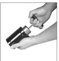
8. Thread the T-Handle, (90.320.1 or 90.320.2), into the end of the piston rod. Pull up on the T-Handle until the rod is extended to its proper stroke length. It may be necessary to use the Valve Bleed Tool, (90.360.4), or the Port Servicing Tool, (90.320.8), to depress the valve to relieve pressure inside the gas spring. **DO NOT** charge the gas spring until the rod is fully extended and the rear head is seated against the c-ring.
