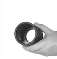
1. Inspect the tube assembly for any damage. Polish out any burrs at the bottom of the tube assembly to avoid damaging seals during the reassembly process. If there are any severe scratches in the finish contact DADCO for repair.
