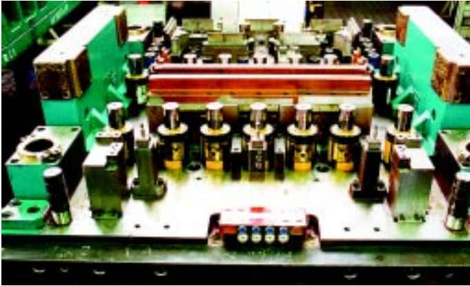
DADCO gas springs are linked to a modular control panel and mounted to an SMS plate. The SMS is secured to the die from the bottom.
