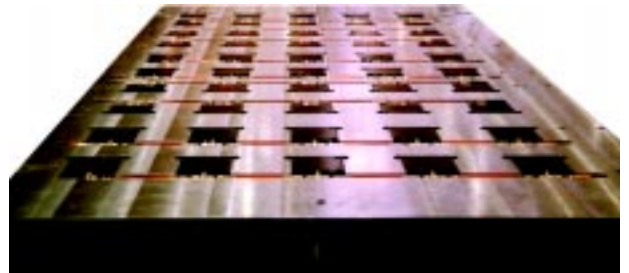
DADCO gas springs are mounted to the SMS from the bottom, for restricted shut height applications.
